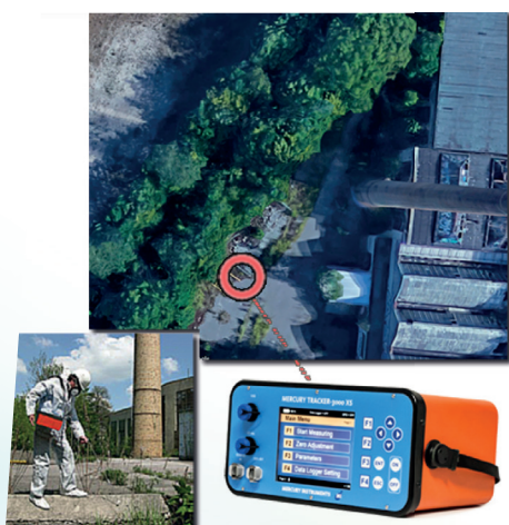
Mercury Tracker-3000 XS: ready for field work with built-in GPS and datalogger.
