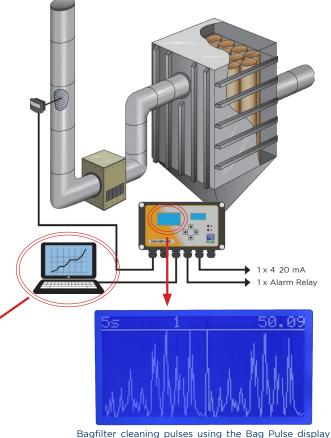
Bagfilter cleaning pulses using the Bag Pulse display on the Control Unit
