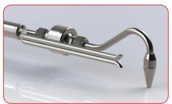
This constructive solution makes the CP2 a versatile and cost effective tool both for flue gas velocity/flowrate evaluations and constant flow or isokinetic sampling in ducts where a standard probe cannot be easily used because of their size.
